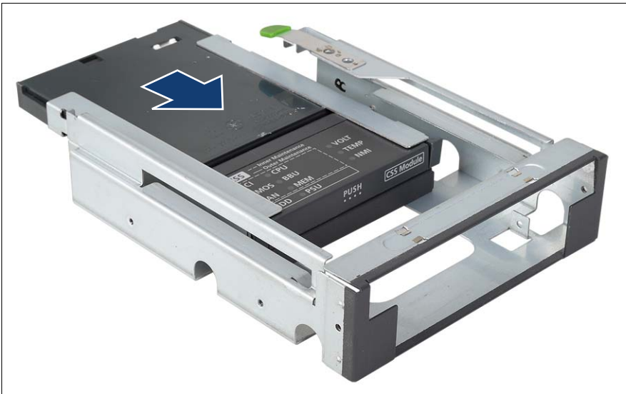
Figure 31: Sliding the 3.5-inch frame with LSP in Multibay 1
